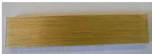
Figure 2. PLLA/sisal fiber unidirectional composite (100 x 15 x 1 mm). [Color figure can be viewed in the online issue, which is available at wileyonlinelibrary.com .]
