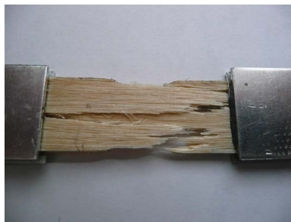
Figure 6. Failed tensile test specimen. [Color figure can be viewed in the online issue, which is available at wileyonlinelibrary.com .]
