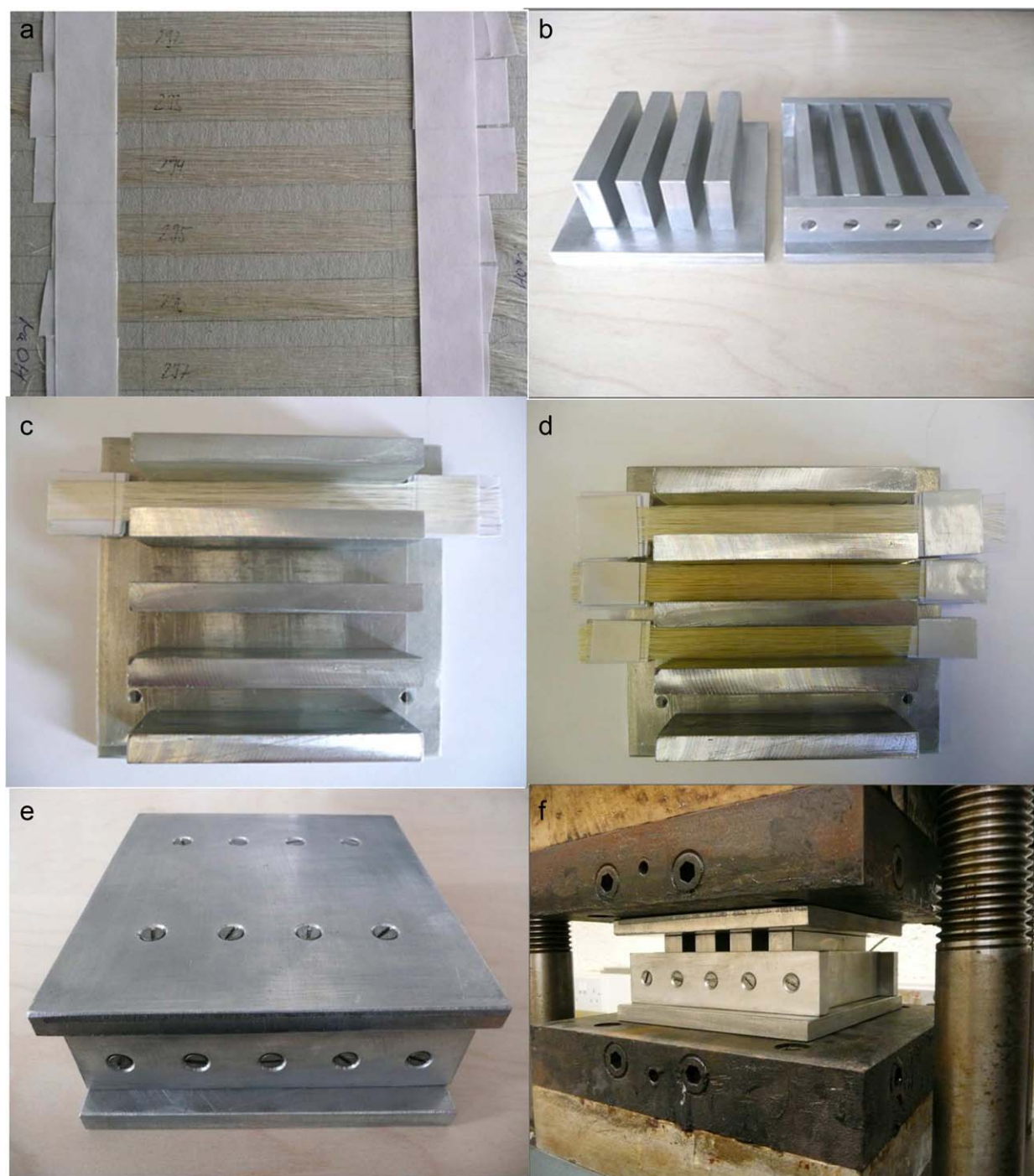
Figure 1. (a) Fiber preforms - aligned untreated sisal fibers glued onto a supporting paper card; (b) Opened compression mold showing the upper clamping part of the mold; (c) Arranging fiber preforms into a mold slot; (d) Combining fiber preforms with polymer foils; (e) Closed mold after consolidation prepared for hot pressing; (f) Mold transferred into a hot press. [Color figure can be viewed in the online issue, which is available at wileyonlinelibrary.com .]
